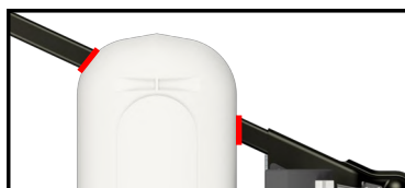
FIGURE C1: Top of A-frame with propane tank cover.
