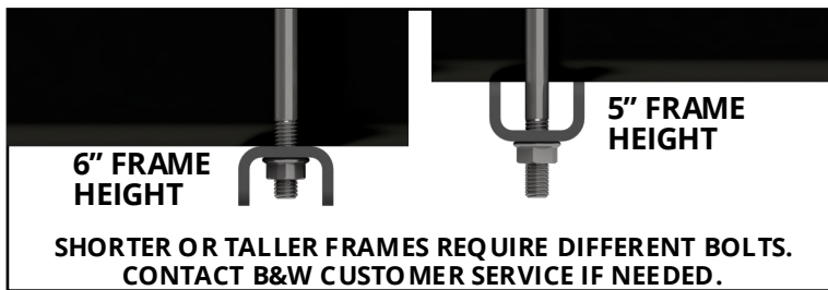
FIGURE D5: View of the frame clamps below the frame.
