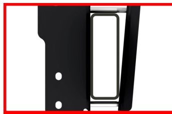
FIGURE C7: View showing an incorrectly tightened inside clamp.
